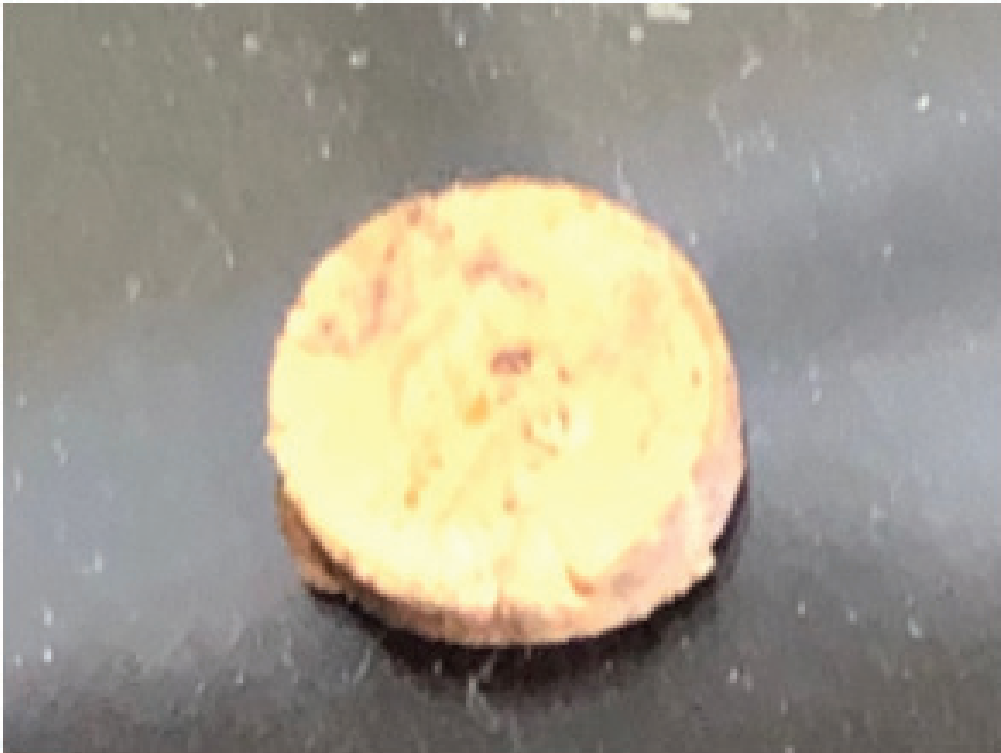
Fig (1-3) disc of gutta percha (0.035 grms) with 5mm width and 2mm height.
